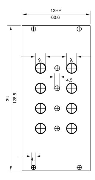
All measurements in millimetres
